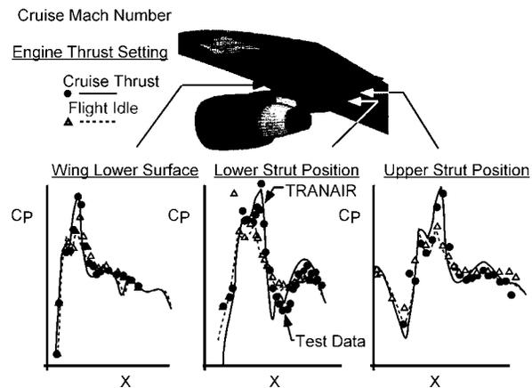
Figure 16. CFD Simulation of Installed Engine Exhaust Effects
