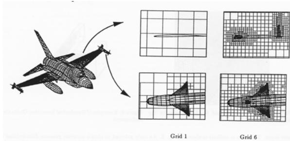
Figure 14. TRANAIR Grid Refinement, Contract Test Case
