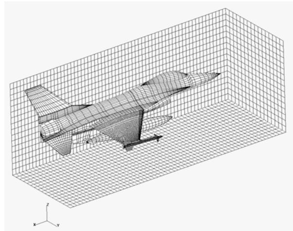
Figure 13. TRANAIR Global Grid, Contract Test Case
