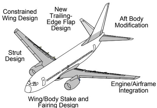
Figure 2. Effect of CFD on the Next Generation 737
