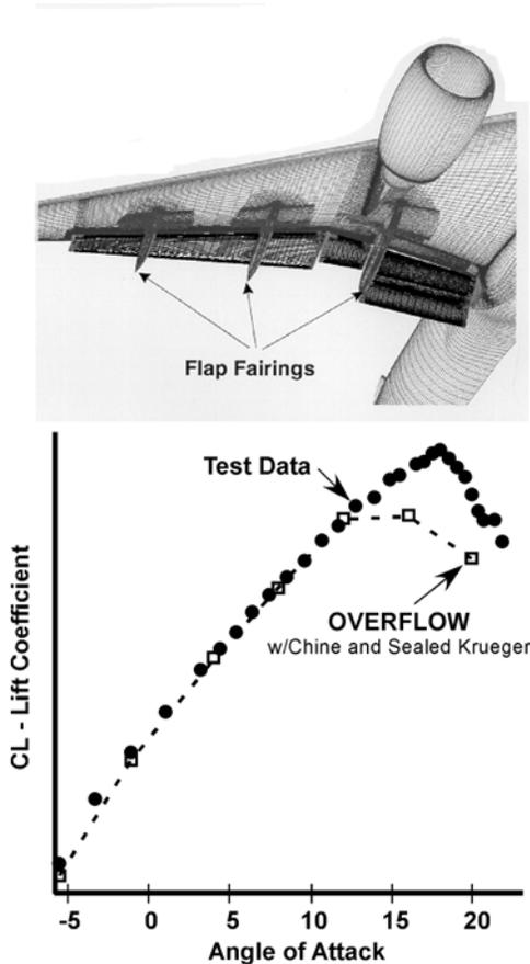
Figure 21. OVERFLOW Solution on a High-Lift Configuration
