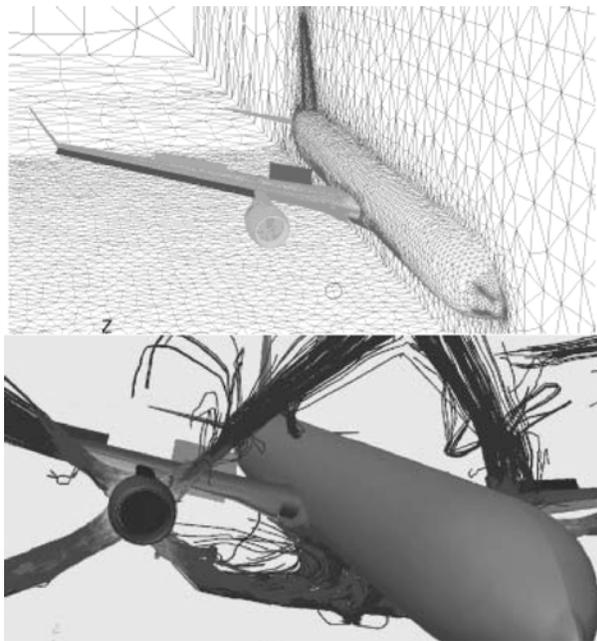
Figure 22. Gridding and Engine Efflux Particle Traces
