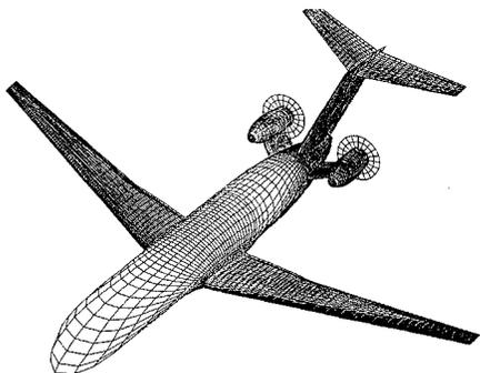
Figure 17. Surface Grid on an Advanced Propfan Transport
